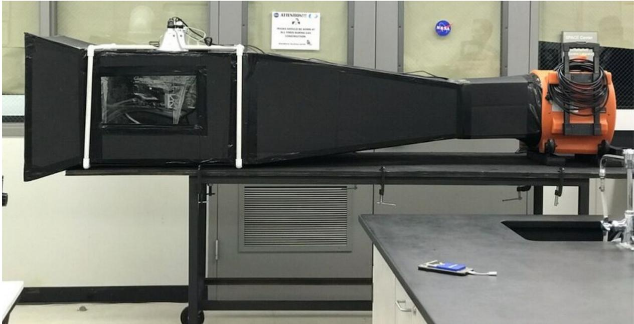
**Figure 26.** Completed Wind Tunnel
