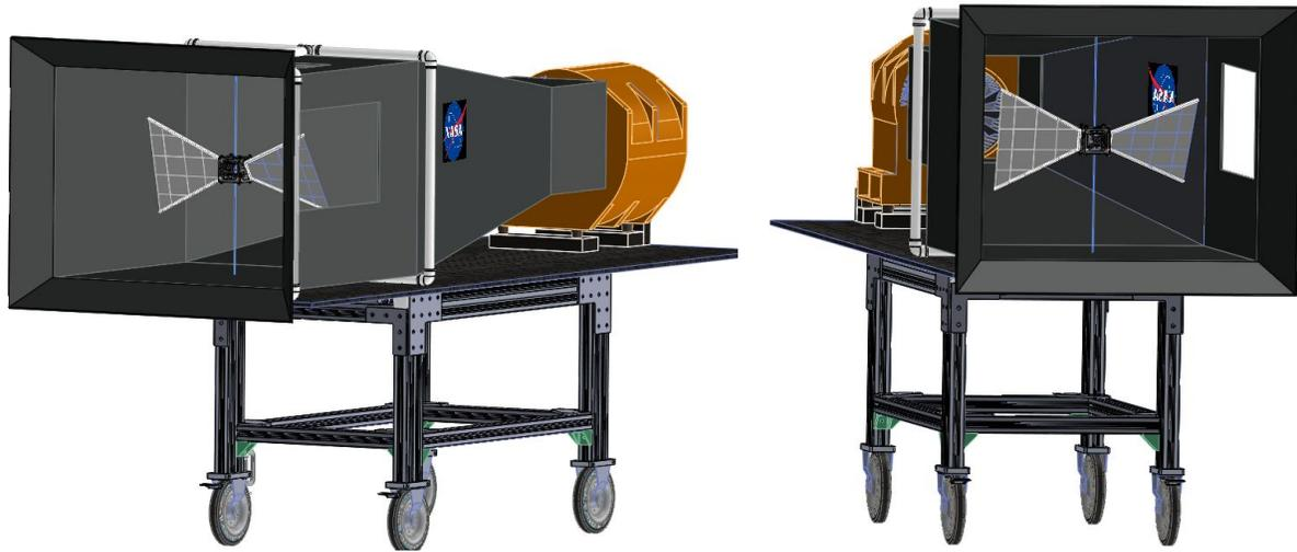
**Figure 24. Wind Tunnel CAD Model Front Views**
